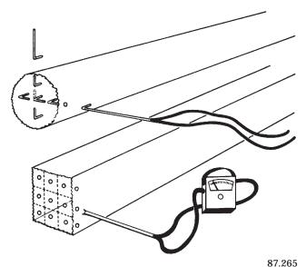
Figure 13-15.—Velocity pressure measurement.
