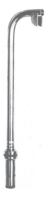
The static pressure probe (fig. 13-8) is used for measuring drops across blowers or fans in duct systems. The probe is carefully placed over an opening in the wall of a duct so as to form a positive seal. The hole should not be less than one-quarter inch in diameter.
