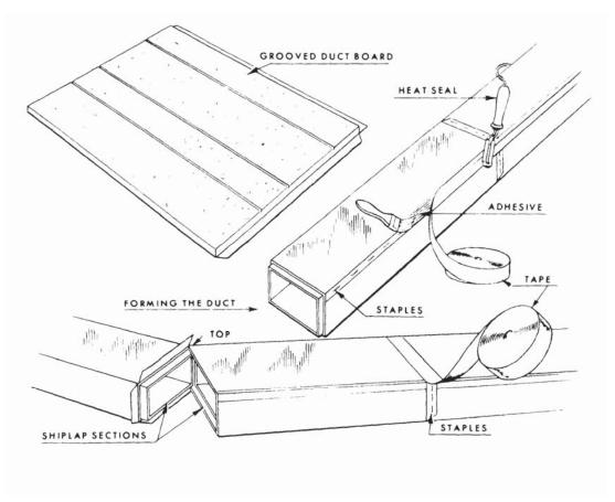
Figure 13-3.—Forming rectangular fiber glass ducts from duct board.
