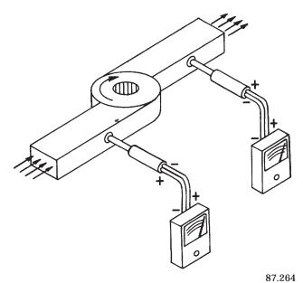
Figure 13-14.—Fan static pressure measurement.
